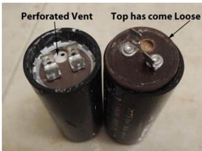
**Testing Capacitors:** This is easy. Buy a cheap capacitor tester off eBay.com and use it. Disconnect the motor and discharge the capacitor with a screwdriver before testing. I test all the capacitors when I am doing an install and whenever there is a problem. The exploded capacitors shown here test to within specifications, but I am discarding them just the same. Caps are cheap compared to motors. I buy replacement capacitors from eBay and from HVAC stores like Johnson Supply.
